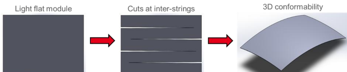
Figure 2.1-4 Conformable PV module design from light flat module to 3D conformability.
