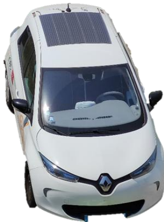
Figure 2.1-5 Global view of a Renault Zoe vehicle with 145 Wp module on roof top.
