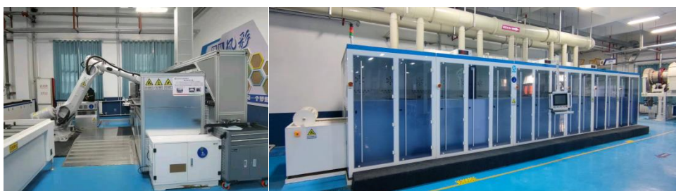
Fig. 2.2-8 State Power Investment Group company self-developed module recycling equipment
