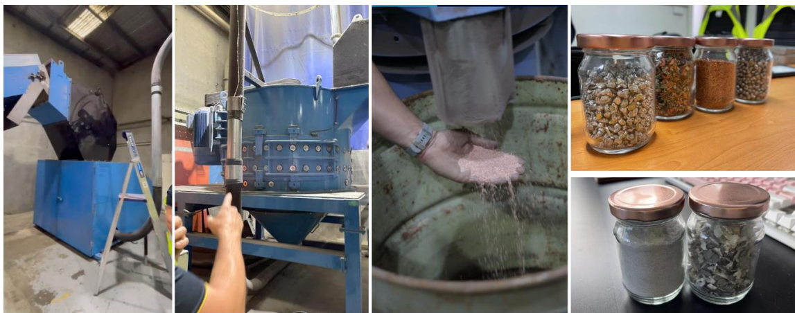
Fig. 2.2-17 Lotus Energy Recycling's crushing and milling technology; recovered products on the right
