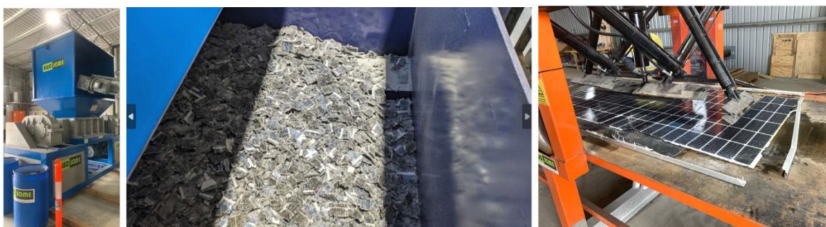
Fig. 2.2-13 Pictures of Elecsome PV recycling operation and products during recycling
