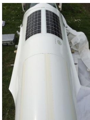
Fig. 10.4-5 The DG 808 of the author with PV integrated in the fuselage (Source: Muntwyler)
