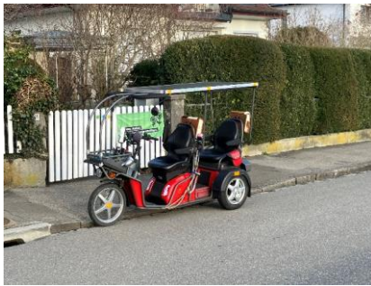
Fig. 9.5-1 Kyburz 3-wheeler with PV (Source: Muntwyler)
